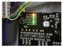
5. Hook a wire to the PWR terminal. You will have multiple wires connected to the PWR terminal. Hook the other end of the wire to a constant 12-volt source (preferably the genset battery, or B+ charger terminal in the transfer switch.) Ensure a proper battery ground at the GND terminal.
