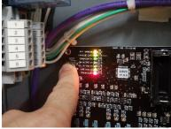
4. Confirm that the common alarm indicator has extinguished. If it does not, repeat the procedure. If it still does not extinguish after repeating, check for other outstanding alarms, such as analog or digital faults. Also, verify that you are running the correct firmware (1.05 and up.)
